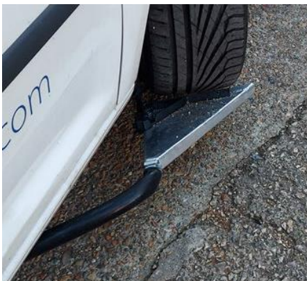
Figure 14 Variants of devices on vehicles for drawing in and measuring particles produced by tire wear in case of road tests, a) first variant, b) second variant, c) third variant [36, 37, 38]
